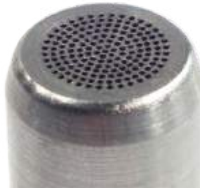
Drilling of holes in the filter - 163 holes \varnothing 0,45 \pm 0,05
