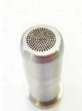
Drilling of holes in the filter - 163 holes \varnothing 0,45 \pm 0,05
