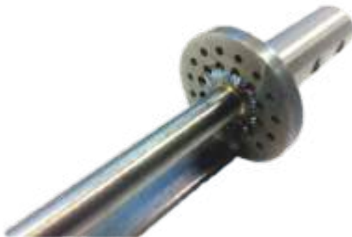
Precise 4-axis welding of the medical implant
